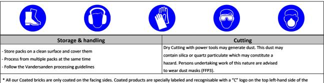
\* All our Coated bricks are only coated on the facing sides. Coated products are specially labeled and recognisable with a "C" logo on the top left-hand side of the packaging. Always check if using coated or non-coated bricks. Match the mortar to the specified initial water absorption.
